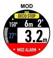
MOD is the maximum allowable depth of the current breathing gas as determined by PPO2 limits.
