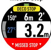
Alarm appears when ascend above the deco stop ceiling depth.
