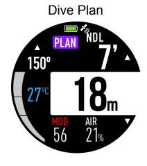
Press button B and button C to change the plan depth to see the allowable NDL.
